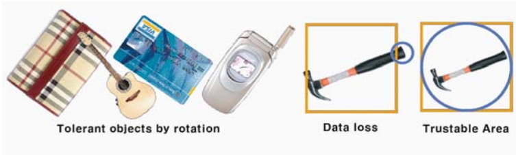
Fig. 5. Left images show examples of Tolerant Objects by rotation. Right image shows data loss by rotation. The object should be in the inscribed circle area in the cell to prevent any data loss by truncation.
