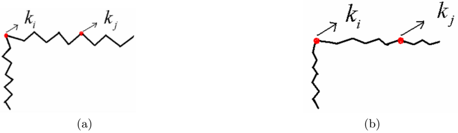
Fig. 2. (a) Original noisy curve, (b) smoothed curve. It can be seen from the illustrations that shape operator defined on the smoothed surface is more accurate.
