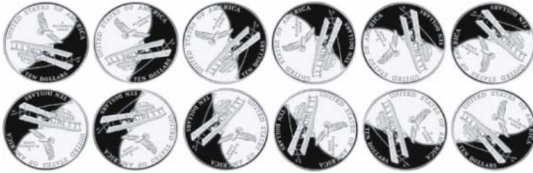
Fig. 4. Rotation of a coin image. Sampling rate is 30 degree. It produces 11 more images from the original image.
