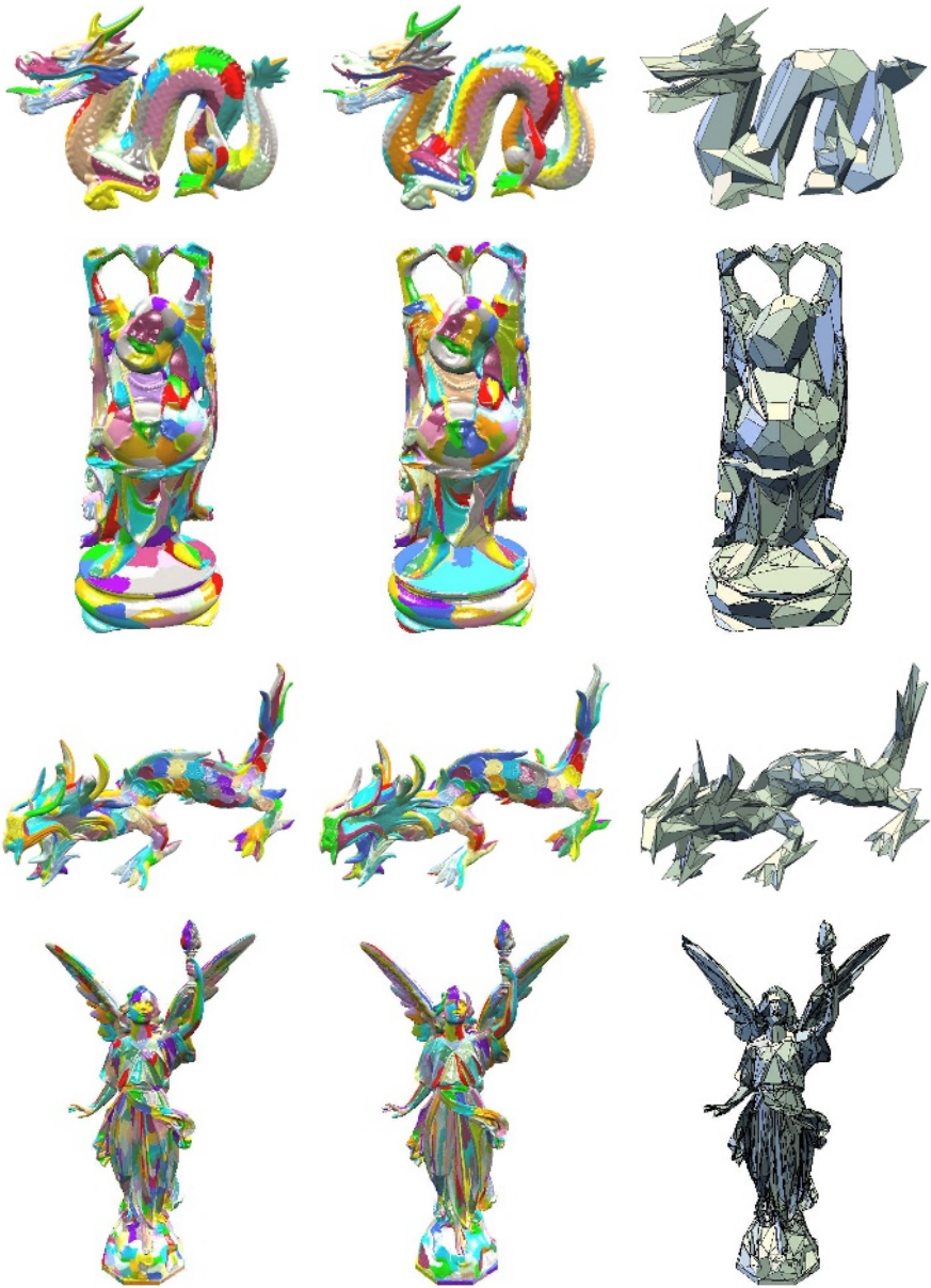
Fig. 5. Chartification and shape approximation results: The first column shows the chartification results for compression, the second column shows the chartification results for shape approximation, and the third column shows approximation meshes
