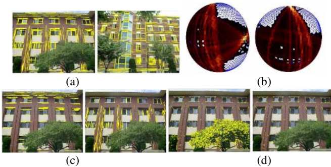
Fig. 2. Result of features extraction: (a) Results of line segments extraction ( \epsilon_d=3, \epsilon_c=0.6 ) (b) Horizontal VP and Vertical VP (the accumulated cells in a Gaussian sphere.), (c) Result of Result of (b), and (d) Harris corners (left) and Corners on façade (right)
