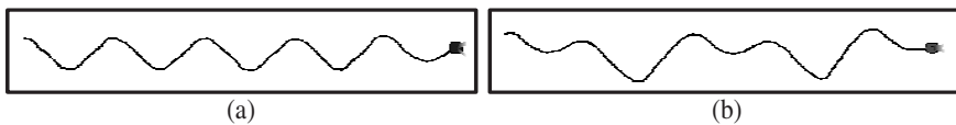
Fig. 3. Paths followed by agents using different equations that control the behavior vector \mathbf{v} : (a) \mathbf{v} = (1, \sin(\omega * t)) ; (b) \mathbf{v} = (1, \sin(\omega * t) + \sin(\omega/2 * t)) , with \omega = \pi/18 and t the current simulation step
